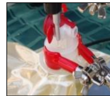
Headspace Oxygen Measurement with optical instrument
