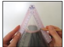
Headspace Volume Measurement with BIB Cone Meter
